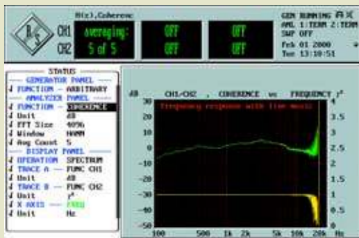
Fig. 13: Transfer and coherence function for determining the transfer characteristic with the aid of complex test signals (e.g. music or voice).
